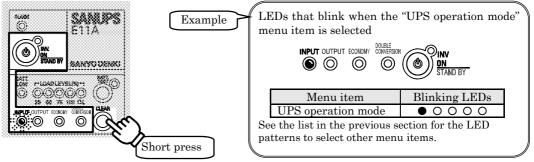
(4) Select the value to set by using the 4 LEDs surrounded by \_\_\_\_\_\_ in the following figure.
